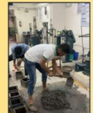
Figure 3. Mixing of concrete
