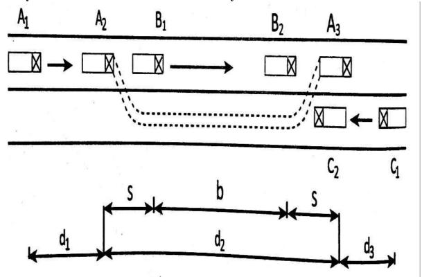
From A1 to A2, the distance 'd1' (m) travelled by overtaking vehicle A at reduced speed 'vb' (m/s) during reaction time 't' (sec),
