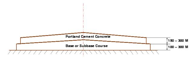
In rigid pavement, load is distributed by the slab action, and the pavement behaves like an elastic plate resting on a viscous medium
