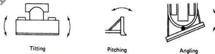
Figure 4-7 Common types of dozer blades.
