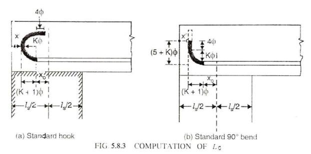
(a) **Case-I : Standard Hook at the end [Fig-5.8.3(a)]:-** The dark portion shows the hook which has an anchorage value of 163 ( IS 456: 2000) for all types of steel. The distance of the beginning of the hook from its apex of the semi circle is equal to (K+1)3 . For mild steel bars K=2 and for HYSD bars, K=4, Hence the distance 3 for mild steel and 53 for HYSD bars. Let *l* be the width of the support.
