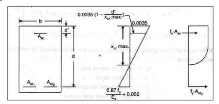
The lever arm for the additional moment of resistance is equal to the distance between the centroids of tension and compression reinforcement, (d - d').
