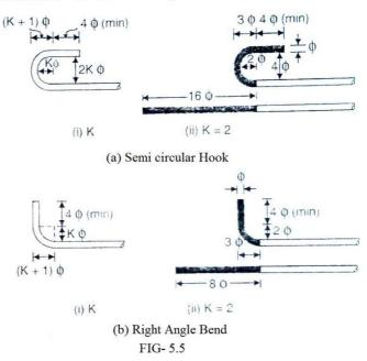
cold twisted steel bars for concrete reinforcement), K is taken as 4. In the case of bars above 25 mm, however, it is desirable to increase the value of K to 3, 4 and 6 respectively.
