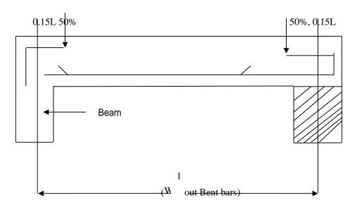
(Typical details of simply supports slab)
