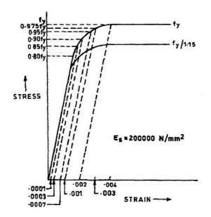
Cold Worked Deformed Bar
