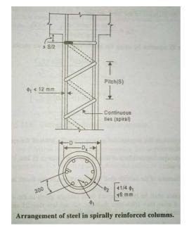
Taking  $A_k$  as the area of the core and  $A_g$  as the area of cross section and using the same assumption about the action of the spiral as is used in the elastic design, the relationship at failure is given by
