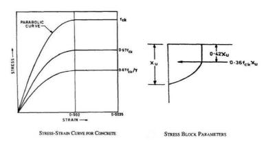
For design purposes, the compressive strength of concrete in the structure shall be assumed to be 0.67 times the characteristic strength. The partial safety factor  $\gamma_m = 1.5$  shall be applied in addition to this.
