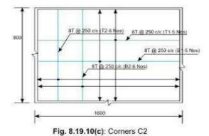
Fig. 8.19.10: Torsion reinforcement bars of Problem 8.2
