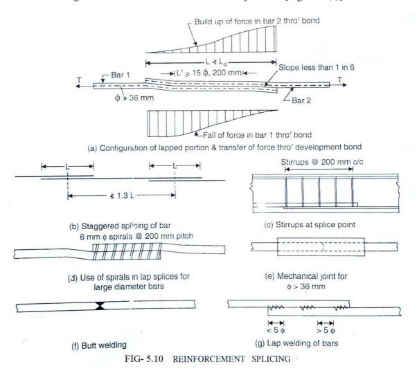
Slicing of a bar is essential in the field due to either the requirements of construction or non availability of bars of desired length. The Figures given are as per the recommendation of the IS 456: 2000.
