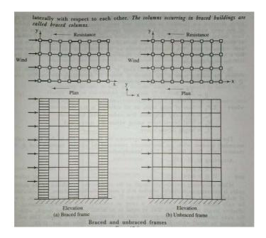
(2) <u>Unbraced columns</u>: A unbraced frames no special bracing systems are provided to resist horizontal forces. In other words the sidesway or joint translation do occur in such columns. The columns shall have to be designed to resist the lateral loads. The column those occur in the buildings where the resistance to lateral loads is provided by the bending in the columns and beams in that plane are called unbraced columns.
