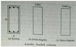
The code adopts the critical value of 0.75  $f_y$  for all grades of steel for finding out the pure axial load carrying capacity of the column. Accordingly
