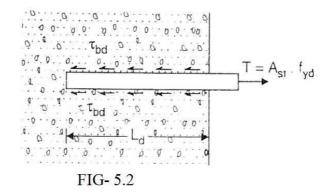
Let us assume that average uniform bond stress is developed along the length. The required length necessary to develop full resisting force is called **Anchorage length** in case of axial tension or compression and **development length** in case of flexural tension and is denoted by  $L_d$ .
