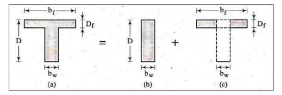
The flanged beam analysis and design are analogous to doubly reinforced rectangular beam. In doubly reinforced beams additional compressive is provided by adding reinforcement in compression zone, whereas in flanged beams, this is provided by the slab concrete, where the spanning of the slab is perpendicular to that of beam and slab is in compression zone.
