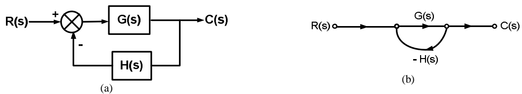
Fig.7.2. (a) Block diagram of a feedback control system and (b) SFG of a feedback control system
