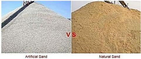
Artificial sand, also called crushed sand or mechanical sand, refers to rocks, mine tailings or industrial waste granules with a particle size of less than 4.75 mm, which are processed by mechanical crushing and sieving, but does not include soft and weathered granules.
