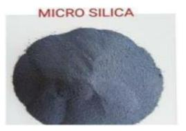
Micro silica or silica fume is an excellent admixture for concrete as it leads to better engineering properties. It reduces thermal cracking, improves durability, and increases strength. Silica fume concrete has a number of construction applications.
