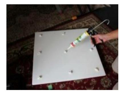
Construction adhesive is a general-purpose adhesive used for attaching drywall, tile, moulding, and fixtures to walls, ceilings, and floors. It is most commonly available in tubes intended for use.
