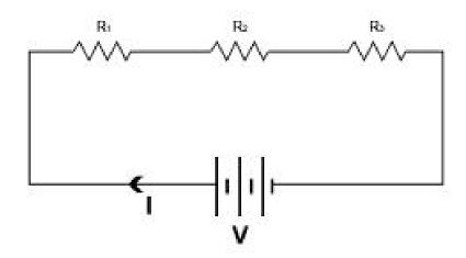
Consider a group of resistances  $R_1$ .  $R_2$  .  $R_3$  are connected in series.
