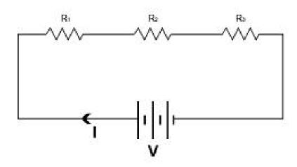
Consider a group of resistances  $R_1$ .  $R_2$  .  $R_3$  are connected in series.
