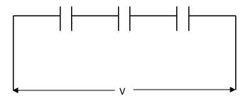
Let Q be the charge of each capacitor, If  $V_1$ ,  $V_2$ ,  $V_3$  are the potential difference across the capacitors respectively
