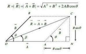
The parallelogram law of vector addition states that if two vectors are represented by the adjacent sides of the parallelogram taken in the same order then the resultant vector is represented by the diagonal passing through the common point taken in opposite order.
