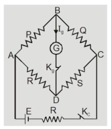
It is an electric arrangement of four resistances connected in the form of a bridge.
