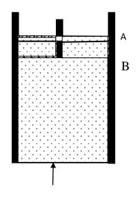
Consider some gas is taken in a barrel having insulating walls and conducting bottom. It is also provided with an insulating piston.
