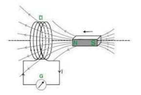
a) Whenever there is a change in magnetic flux linked with a circuit or a coil, an e.m.f. is induced.
