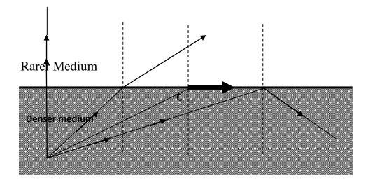
When the ray of light moves from denser to rarer medium, if the angle of incidence is greater than the critical angle , the ray reflected back to the same medium .This phenomenon is known as total internal reflection.
