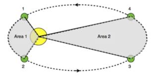
When a planet revolves around the sun it sweeps out equal area in equal interval of time
