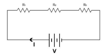
Consider a group of resistances  $R_1$ .  $R_2$ .  $R_3$  are connected in series.
