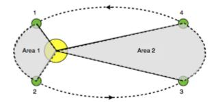
When a planet revolves around the sun it sweeps out equal area in equal interval of time
