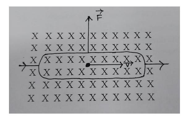
The force  $d\vec{F}$  by this charge is given by,  $d\vec{F} = dq(\vec{v} \times \vec{B})$  If the charge travels a small distance  $d\vec{l}$  in a small time dt, then  $\vec{v} = \frac{d\vec{l}}{dt}$
