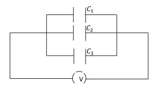
Let V be the potential difference between two plates of each capacitor.
