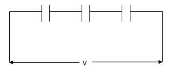
Let Q be the charge of each capacitor, If  $V_1$ ,  $V_2$ ,  $V_3$  are the potential difference across the capacitors respectively
