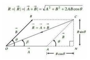
The parallelogram law of vector addition states that if two vectors are represented by the adjacent sides of the parallelogram taken in the same order then the resultant vector is represented by the diagonal passing through the common point taken in opposite order.
