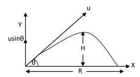
Consider a projectile fired making an angle  $\theta$  with horizontal, with a velocity u.
