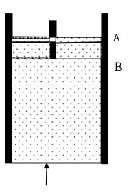
Consider some gas is taken in a barrel having insulating walls and conducting bottom. It is also provided with an insulating piston.
